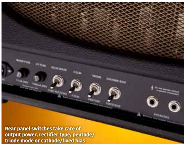
Rear panel switches take care of output power, rectifier type, pentode/triode mode or cathode/fixed bias
